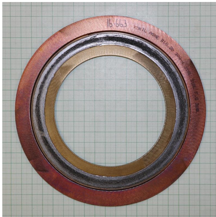
Shell leakage test (T) according MESG SPE 85/300 - 3.3.2
